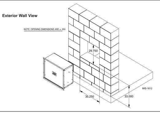
NOTE: Wall opening and wall sleeve required only when one of the ventilation options is utilized. Installations not utilizing any ventilation option can be made in any interior space accessible to electrical supply, water supply system and condensate drain.
