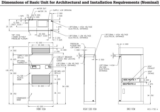
NOTE 1: Ventilation intake opening for barometric fresh air damper, commercial room ventilator (CRV) or energy recovery ventilator (ERV). Opening is sealed if no vent option.
